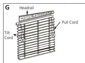
**G.** Always tilt blind horizontally before raising/lowering to extend the life of the blind. **To lower blind:** Move cord to left pulling down gently until cord lock releases. **To raise blind:** Pull cord downward until blind reaches desired height. **To lock cords:** Pull cord right and release. Cord will lock automatically.
