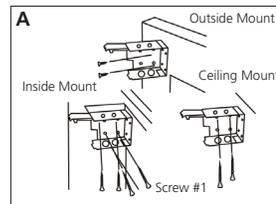
**A.** Brackets should be placed at the width of blinds headrail 6mm past each end. The bracket doesn't necessarily need to touch the inside face of the window frame.
