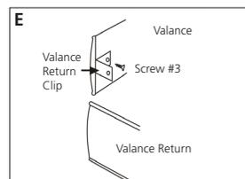
**E. For Outside Mount:** Screw one end of the valance return clip onto the valance using Screw #3. Align the edge of the valance return with the valance. Screw the other end of the valance clip onto the valance return.
