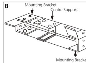
**B.** Align the top of the centre support bracket with the top of the mounting bracket before installation. Install with the bigger flap of the centre support bracket on the top side and clear of the slat ladder positions.
