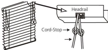
1. Install blind as directed by manufacturer making sure headrail is securely fastened. Lower blind to maximum desired length and lock into place.
