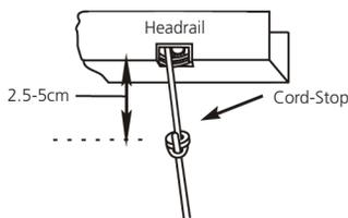
4. Push both the cord-stop and the loosened knot toward the headrail until the cord-stop is 2.5cm to 5cm below the headrail. Hold cord-stop in place and pull firmly on lift cord to re-tighten knot. Repeat steps 2, 3 & 4 for each cord-stop.
