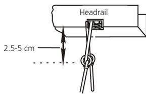
2. Measure the distance from headrail to cord-stops. If cord-stops are 2.5cm to 5cm below the headrail no further adjustment is needed. Your blind is ready to be used.
