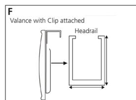
**F.** Hook valance clip with valance attached onto the top of the headrail.
