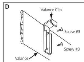
**D.** Screw valance clips onto back side of the valance with screws provided (Screw #3)
