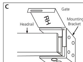
**C.** Push rail into brackets. Then press gate to close brackets.
