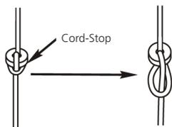
3. If cord-stops ARE NOT 2.5cm to 5cm below headrail loosened (but do not untie) the knot surrounding the cord-stop.
